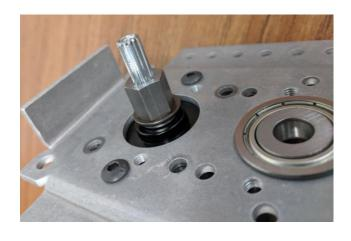
Step 4c: Place one 8mm brown washer and then two 1/4 in. thick Falcon 500 shaft spacers over the shaft to bring it flush to the top. These spacers were included with your Falcon 500.
