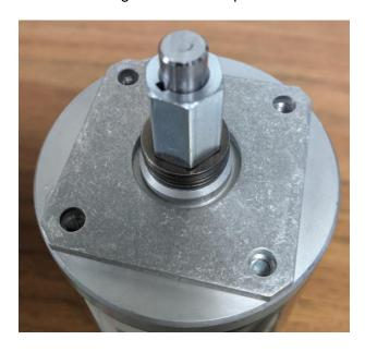
**Step 4a:** Slip your pinion gear over the hex adapter. If you want the gearbox to spin faster than the motor put the larger of the two gears here. If you want it to spin slower, but with more torque, put the smaller gear here.
