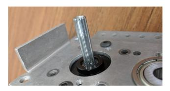
**Step 3c**: Slip your pinion gear over the hex adapter. If you want the gearbox to spin faster than the Falcon 500 motor put the larger of the two gears here. If you want it to spin slower, but with more torque put the smaller gear here.
