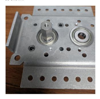
Step 4b: Place the pinion gear onto the 1/2 in. hex shaft then place the other 1/4 in. spacer (am-3948-250) over the gear to bring the stack flush with the top of the shaft. Again, if your shaft is different, you may need to supply your own spacers. If you want the Flyer Gearbox to spin faster than the Sport, put the larger of the two gears here. If you want it to spin slower, but with more torque put the smaller gear here.
