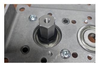
**Step 2b:** Install the 3/8 in. ID bearing (am-0573) in the bearing hole in the plate (am-4216) furthest from the bent tab. The flange of the bearing should be on the same side as the tab. Place this assembly on top of the Sport gearbox as shown.
