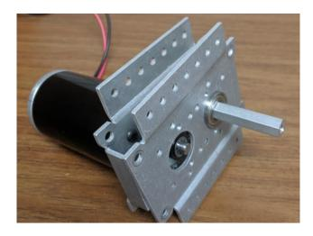
Step 7d: Flip the gearbox over and before installing the second spacer apply a liberal amount of grease (am-2768) to both gears, spin the shaft by hand to mix the grease around and into all the valleys of the gear teeth. Once greasing is complete, repeat step 6d for the other spacer. Now tighten all bolts while ensuring that the output shaft still spins and that the corners of the spacers line up with the gearbox plates.
